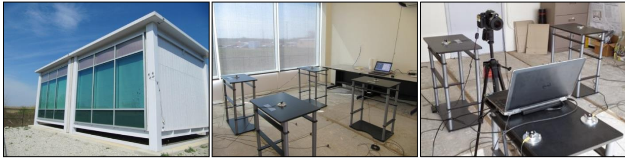
Fig. 2. Exterior view of test offices; interior view; HDR camera for luminance measurements.
