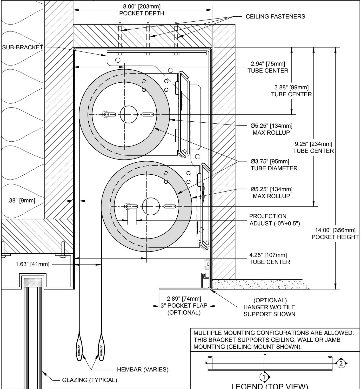
MULTIPLE MOUNTING CONFIGURATIONS ARE ALLOWED: THIS BRACKET SUPPORTS CEILING, WALL OR JAMB MOUNTING (CEILING MOUNT SHOWN).
