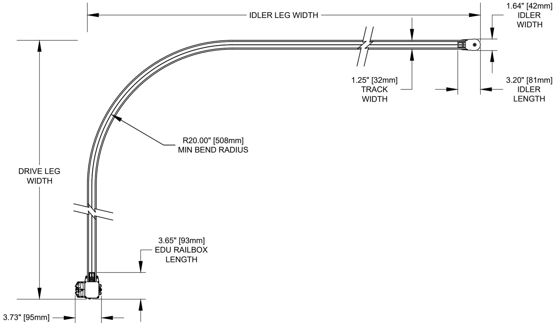
DRAPERY TRACKS INSTALLED AS PROVIDED BY FACTORY PER THIS DRAWING WILL HAVE ALL NECESSARY CLEARANCES FOR PROPER OPERATION OF TYPICAL FABRIC PANELS. IT IS THE RESPONSIBILITY OF THE INSTALLER TO ENSURE PROPER CLEARANCES ARE MAINTAINED BASED ON ACTUAL FABRIC PANEL SELECTION.
