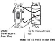
The "COMMON" terminal is the different colored screw (not green) or the terminal marked "COMMON." Tag this wire on each switch to identify it in Step 5.
