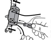
Backwired: Insert screwdriver. Pull wire out.
