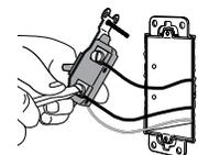
Screw Terminals: Turn screws to loosen.
