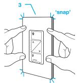
(If you installed the dimmer next to other dimmers or switches, you'll need to install a wallplate with the correct size/number of openings to accommodate all the devices.)
