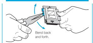
Do not remove outside side sections on dimmers at the end of gang
