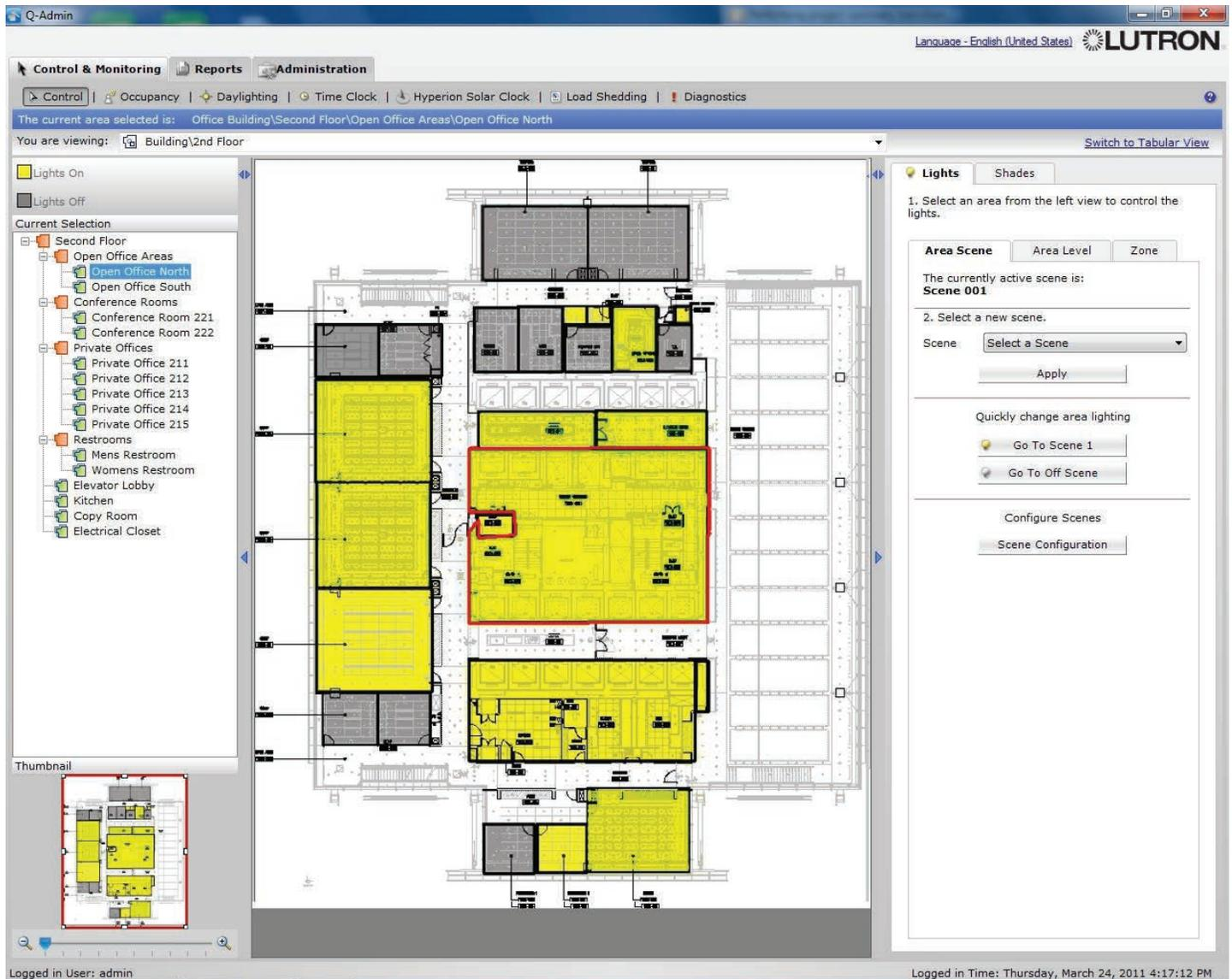
Graphical view allows the user to select/view areas by selecting within a graphical floorplan, as shown.
