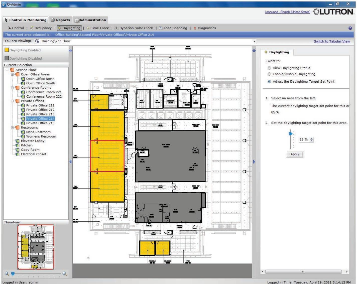
Dimmed daylighting: Daylight set points can be changed for each daylit area. This is particularly useful when new departments with different lighting requirements move into a space. The daylighting target set point for an area ranges from 0 to 100 percent.
