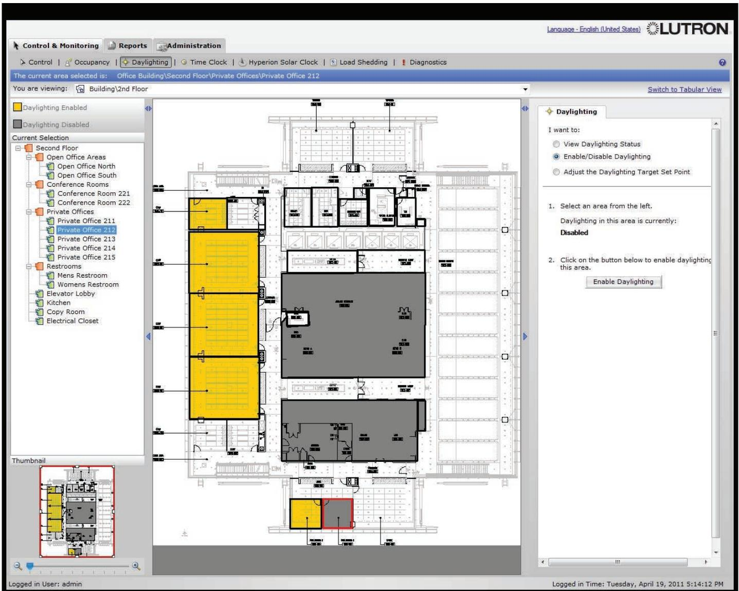
The Daylighting screen allows a building manager to control and monitor daylighting for areas.
