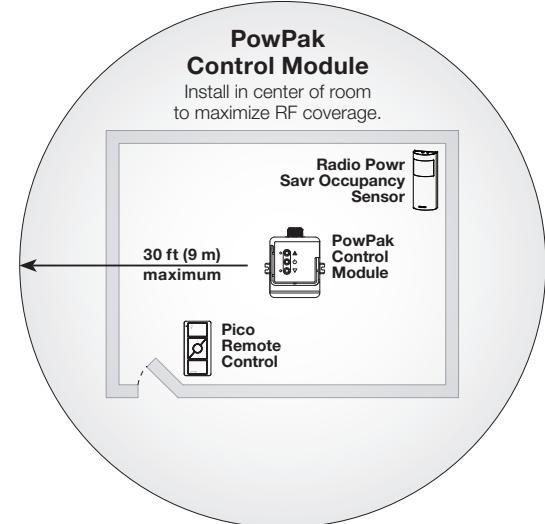
All Wireless Transmitters must be installed within 30 ft (9 m) of the PowPak Control Module with EcoSystem technology.
