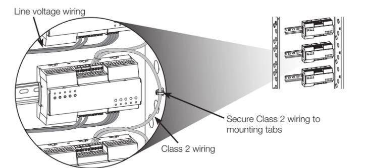
**10. Place end stop and bypass solution in panel.**
