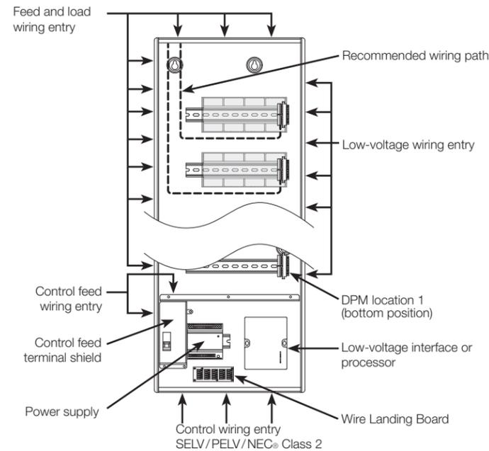
**5. Control feed wiring (control panels only).**
