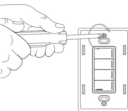
**5 Mount the dimmer and attach the wallplate**
