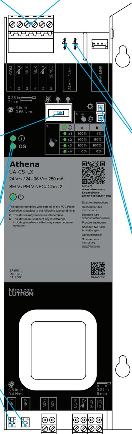
**NOTE:** The power LED should always be lit when power is applied. Do not use the LED as a panel power indicator. Always remove power from the panel before handling terminals or connectors.
