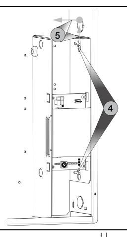
Mount the transformer in the legacy panel using the transformer mounting holes.
