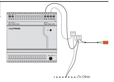
Connect the QS link terminal block (provided) to a QS link from a wired HomeWorks QSX processor that was added to the panel when replacing the 8-series processor with internal module interface link.
