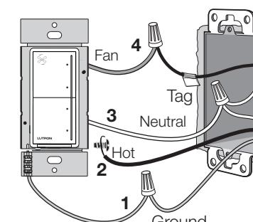
**1** Connect the bare copper (or green) "ground" wire from the wallbox to the green wire on the fan control using a wire connector.
