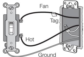
Place tag on fan wire (if unsure, pick one, and if the fan does not work turn power off, and swap wire).
