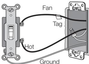
Disconnect all three wires from the switch.
