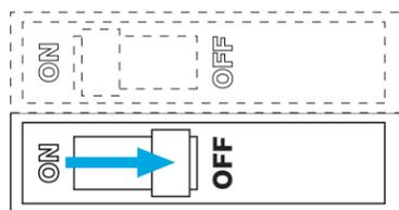
**WARNING: SHOCK HAZARD.** May result in serious injury or death. Turn off power at circuit breaker or fuse before installing.
