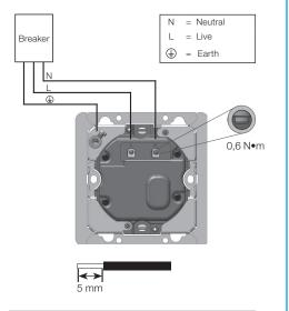
Products must be installed in accordance with the latest building and IEE wiring regulations.
