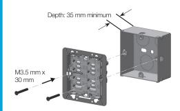
Mount the keypad to the backbox using the horizontally located screw holes only as shown.
