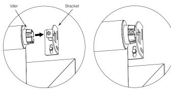
5.2 Depress the spring loaded idler by pressing the shade towards the idler, and install the drive side of the shade onto its bracket.
