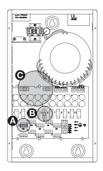
If an output status LED has turned off, the fuse will need to be replaced. The QSPS-P2-10-60 comes with two spare 5x20 mm 2.5 A fuses.
