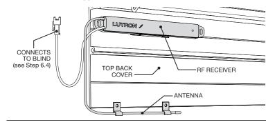
4.2 Using the clips provided with the RF Receiver, secure the antenna so that it hangs below the bottom edge of the Top Back Cover.
