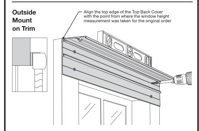
NOTE: The Top Back Cover may also be outside-mounted above the trim. Use spacer blocks (not included) of sufficient thickness to ensure the blind clears the trim
