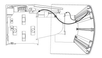
9.3 Press along the lower half of the Fascia near the ends to engage the hooks at the bottom of the End Brackets.
