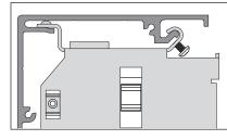
5.3 Center the blind on the window, then tighten the retaining screw on the front hook of each End Bracket to secure the blind in position.
