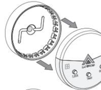
b. Pre-drill a pilot hole, if appropriate, through the hole in the sensor's back cover (and through the adhesive used to mount the sensor in step 3).
