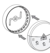
d. Align the sensor with the mounted back cover and gently press it in until it locks in with a click.
