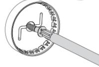
c. Secure the sensor's back cover to the mullion using a #4 flat-head screw of appropriate length and type for the material. Hand-tighten only; **DO NOT** use a power tool.
