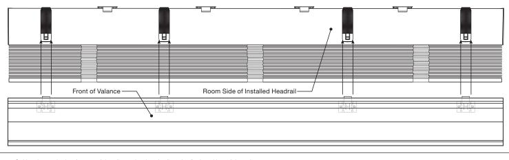
C. Use the ratcheting feature of the clips to level and adjust the final position of the valance.
