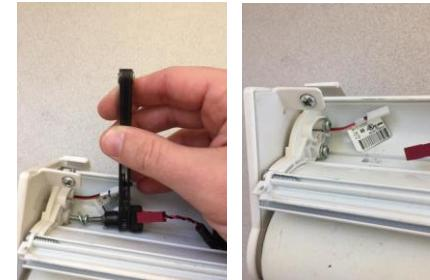
Use 90° T15 (Torx) driver to reinstall battery tray washers and screws.
