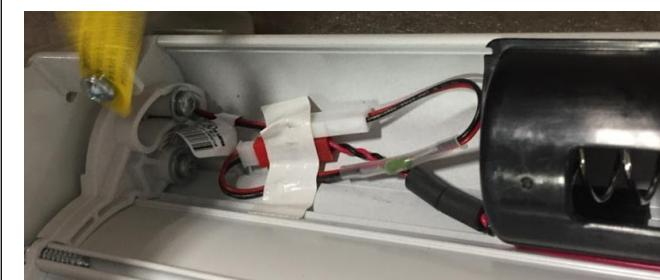
Connect supplied NEW in-line fuse between EDU and battery box.
