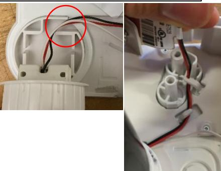
Route white antenna wire in channel. Press wire in at the 6 "teeth" to secure in place.
