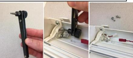
Some shades may contain a spring and spacer at this location. Remove screws in the same way and save all parts, which will be reinstalled later.
