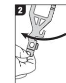
2 Rotate the clip away from the stop as shown.
