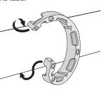
Slide the Lift Ring along the tube, aligning it with a lift cord position.
