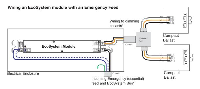
\* Module terminals are compatible with #18 and #16 AWG solid wires only, sensor terminals are compatible with #22 AWG solid only.
