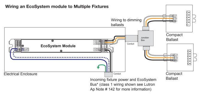
\* Module terminals are compatible with #18 and #16 AWG solid wires only, sensor input terminals are compatible with #22 AWG solid only
