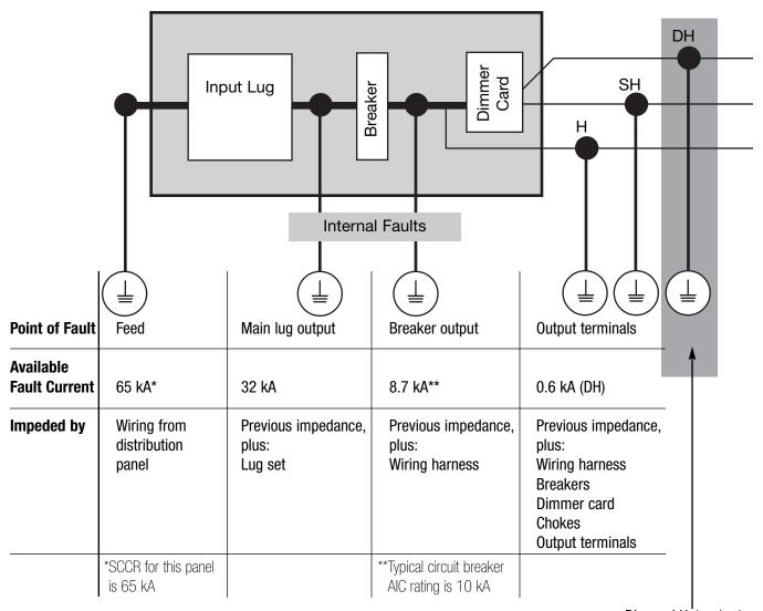
Dimmed Hot output terminal is the typical point at which faults might occur.
