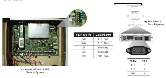
**Note:** Normally RS232 connections would be wired with TXD connected to RXD. In this case TXD is wired to TXD and RXD to RXD so that a Null Modem adapter is not needed.
