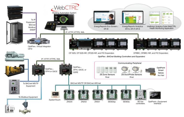
The WebCTRL<sub>®</sub> system's open standards with BACnet native architecture makes integration with other mechanical and electrical building systems simple. BACnet is the global standard for open interoperability. The BACnet protocol is available as an American National Standard, a European standard, and global ISO Standard 16484-6:2014.
