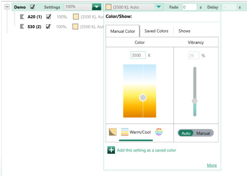
**Figure 20:** Ketra not only allows independent control of intensity and CCT, but also allows a user to adjust vibrancy (maintaining CCT while adjusting the spectral power density to manipulate color reflection in the space).
