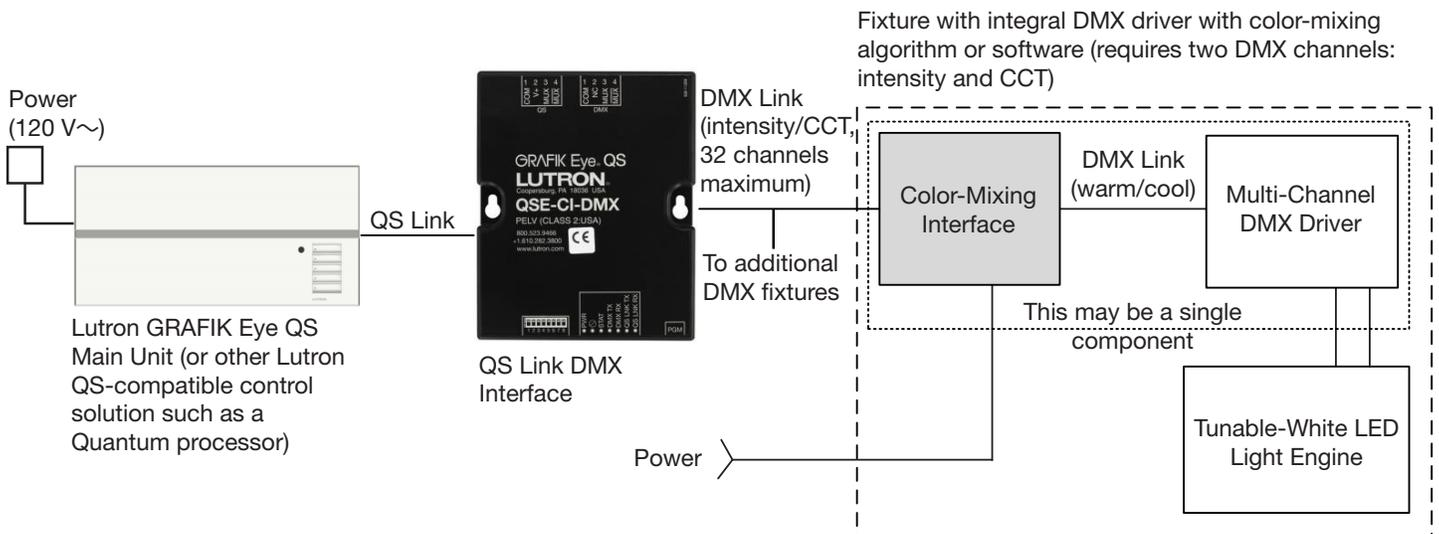
**Figure 17:** DMX providing independent control of intensity and color temperature.
