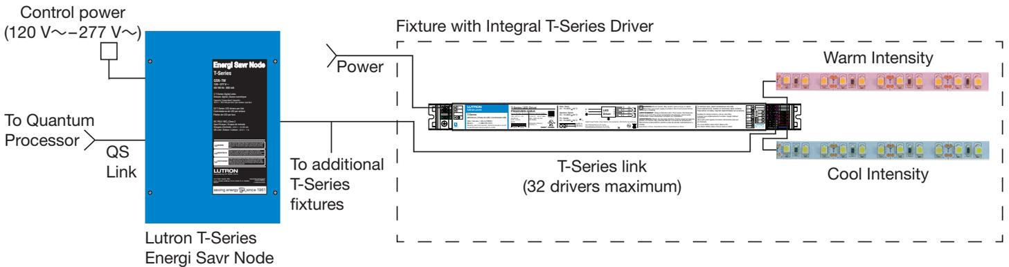
**Figure 13:** Lutron T-Series control and driver providing independent control of intensity and color temperature.
