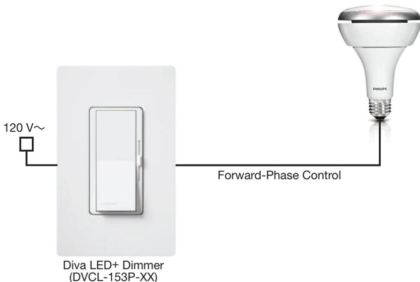
**Figure 4:** Lutron Diva LED+ dimmer controlling Philips DimTone® LED.
