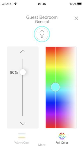
**Figure 24:** Full-Color tuning using saturation/hue is available via the Lutron App.
