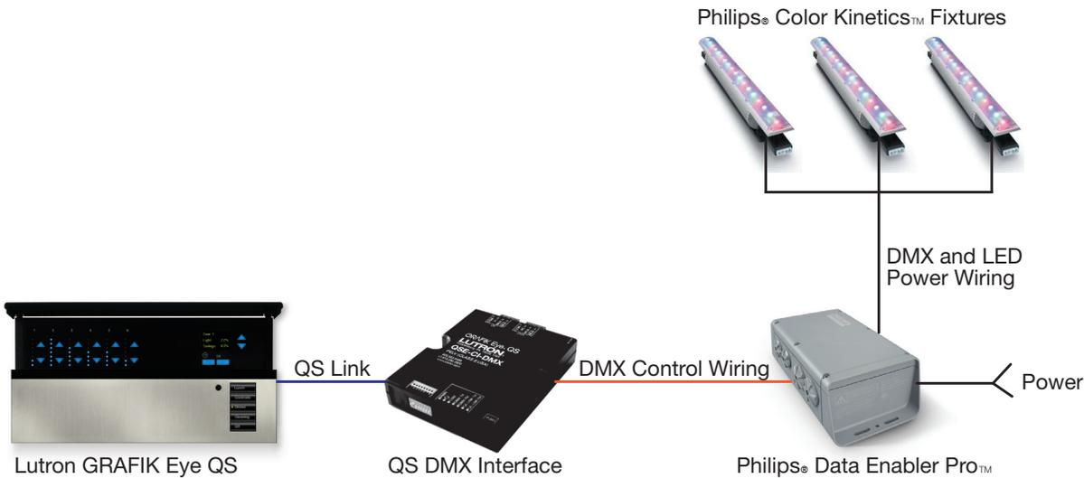
**Figure 23:** Lutron GRAFIK Eye QS unit controlling Philips® Color Kinetics™ fixtures through DMX control.
