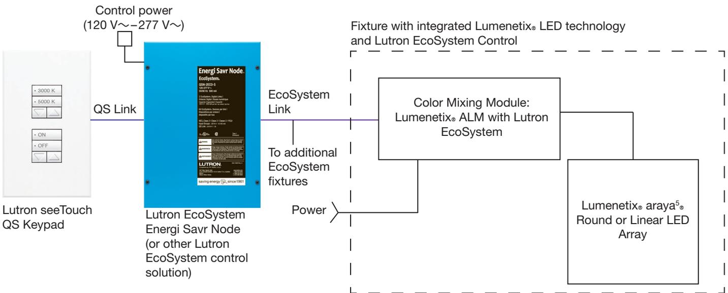
**Figure 16:** Lutron EcoSystem providing independent control of intensity and color temperature.
