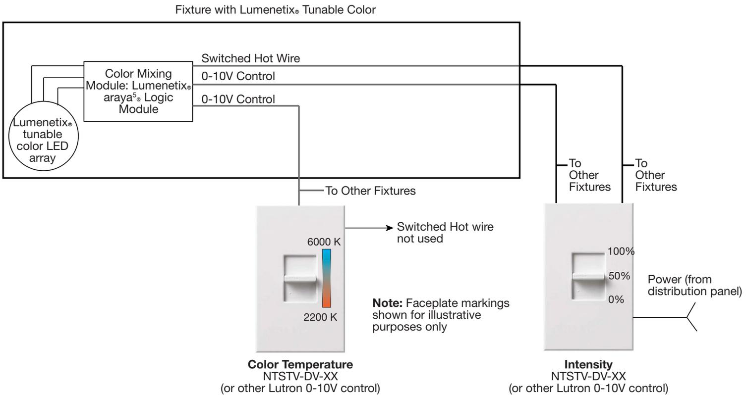
**Figure 14:** Lutron Nova T<sup>☆</sup> slide dimmers providing independent control of intensity and color temperature of a Lumenetix® fixture with a tunable color LED array fixture inside.
