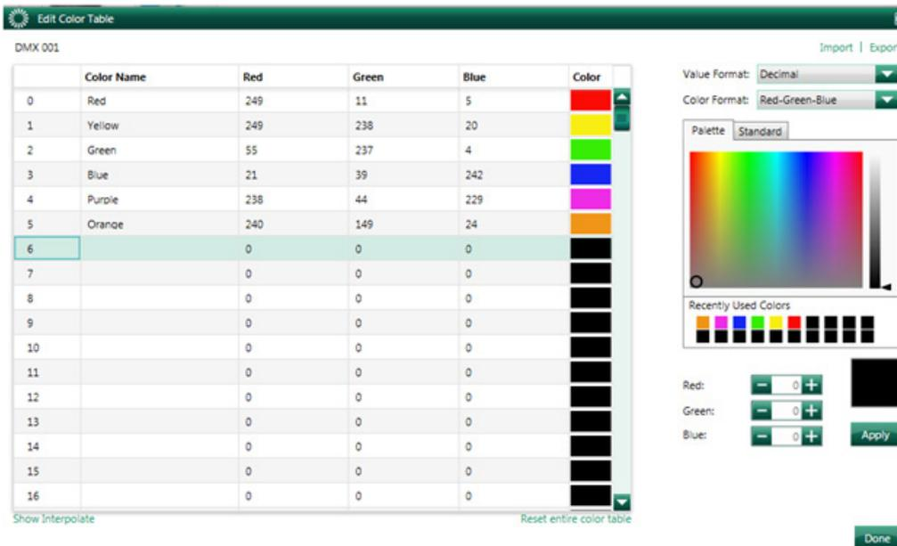
**Figure 25:** Color Table tool for DMX 3 channel lighting control packaged with Lutron Quantum design software.
