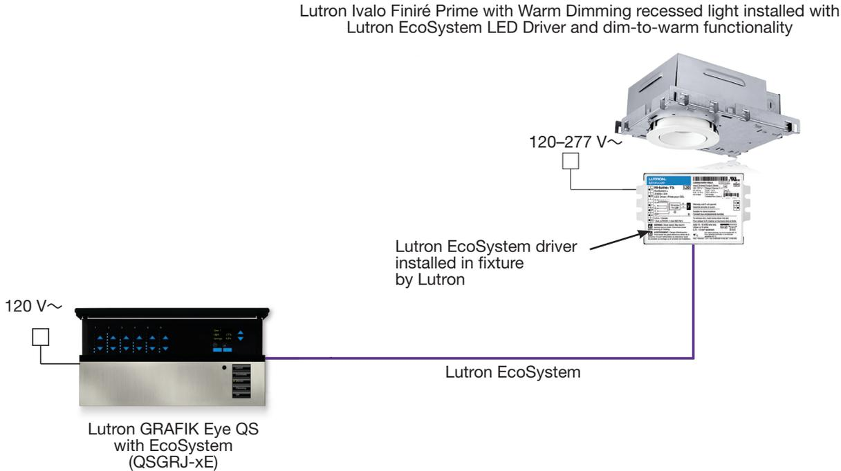
**Figure 5:** Lutron GRAFIK Eye QS unit controlling Lutron Ivalo Finiré Prime with Warm Dimming recessed light installed with Lutron EcoSystem LED driver.
