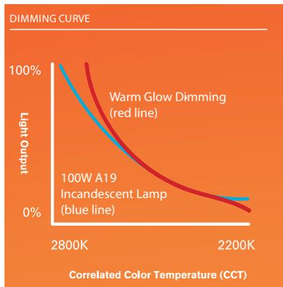
**Figure 3:** CCT curves for incandescent lamp and USAI Lighting luminaire with Warm Glow® Dimming technology.
