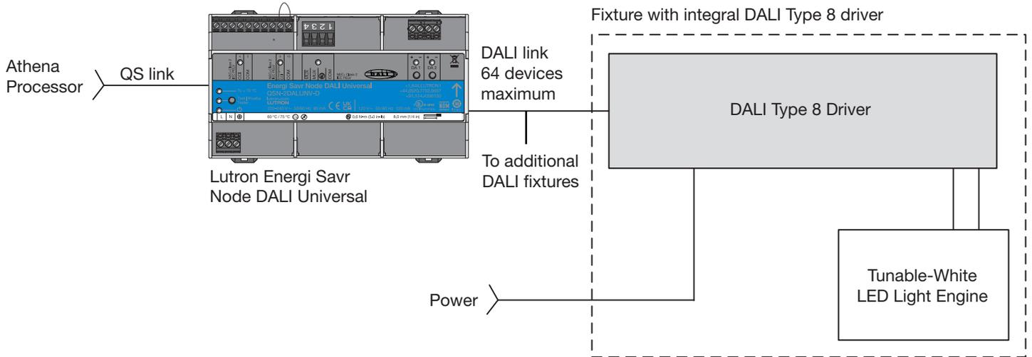
**Figure 19:** DALI Type 8 implementation providing independent control of intensity and color temperature
