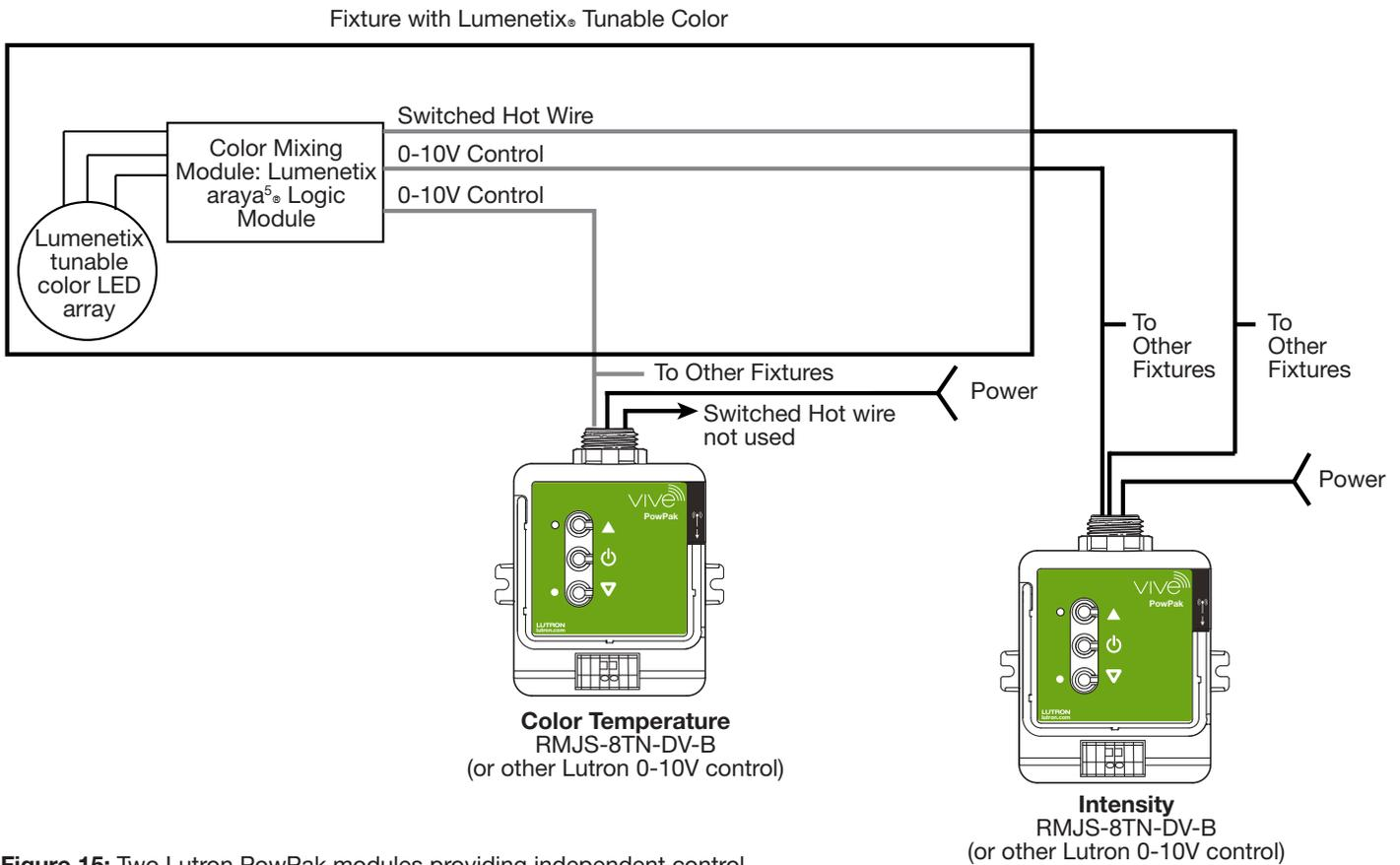
**Figure 15:** Two Lutron PowPak modules providing independent control of intensity and color temperature.
