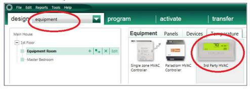
Once the 3rd Party HVAC device has been added to the *Equipment* area, provide a name for the HVAC device and select *Mitsubishi* as the *Manufacturer*.
