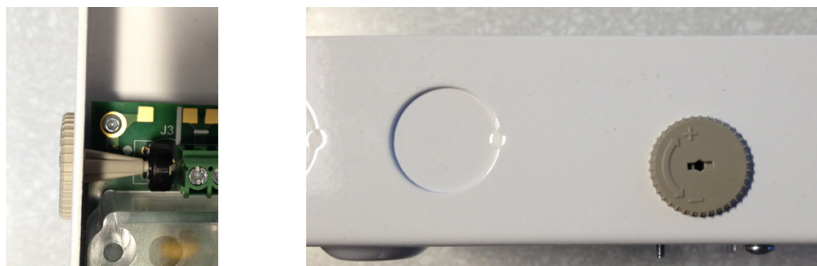
Figure 10. Example of a Field Adjustment Knob on a Lutron Driver
