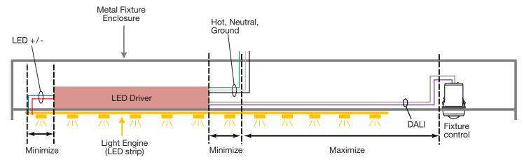
**Note:** If the driver is provided with a ground terminal, this terminal should be electrically connected to the grounded fixture metal as close to the driver as possible.
