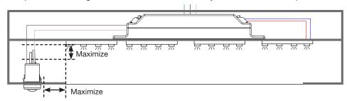
All wires should be routed as far away from the Vive integral fixture control as possible (3 in [76 mm] minimum separation suggested)
