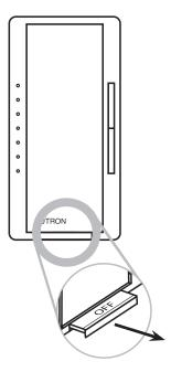
2. Press and hold **\( \Lambda \)**. Close the FASS and continue to hold **\( \Lambda \)** for 5 seconds.
