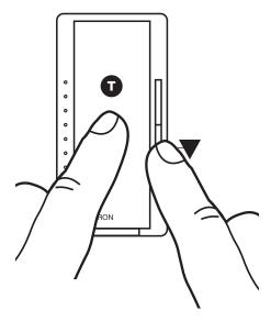
2. Press ▲ or ▼ to adjust light output until stable and not flickering. Press and release **1** to save setting.
