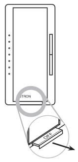
2. Press and hold ①. While continuing to hold ①, push the FASS to the ON position (in) and continue to hold ① for approximately 5 seconds.
