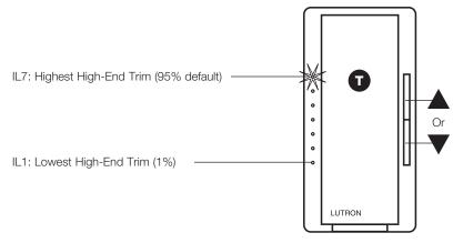
3. **To save** the desired *High-End Trim* setting, **press** 1. This will exit out of the *High-End Trim* option and return to the *APM* main menu.
