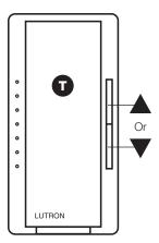
3. Press and release to turn load OFF, then press ▲ once. If load does not turn ON or remains unstable, repeat Step 1 and in Step 2, increase light with ▲.
