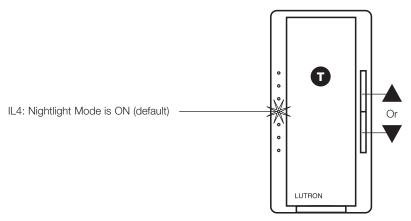
3. **To save** the desired *Enable/Disable Indicator Lights* setting, **press 1**. This will exit out of the *Enable/Disable Indicator Lights* option and return to the *APM* main menu.
