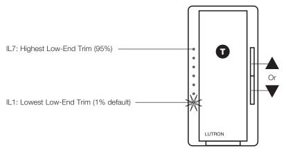
3. To save the desired Low-End Trim setting, press ①. This will exit out of the Low-End Trim option and return to the APM main menu.
