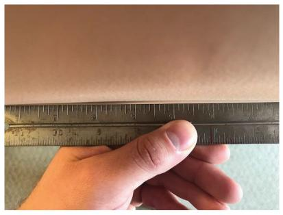
Photo 2: Photo of straight edge used to evaluate wall flatness for Glass Units.
