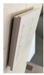
Photo 4: Example of a protruding wallbox and its impact on the keypad.
