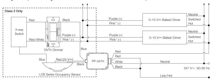
For applications requiring 4-way occupancy sensing and manual control functionality, a DVTV dimmer can be installed as shown below between the sensor and the power pack. Two toggle switches are added to switch the red and red / white line side inputs of the dimmer to provide 4-way functionality. Similar to the previous application, the sensor will turn the lights on upon detecting motion if either of the switches or the dimmer are in the on position.
