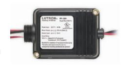
air (plenums). The PP-347H power pack fits inside a standard 4 in x 4 in (102 mm x 102 mm) junction box or standard fluorescent fixture ballast cavity, mounts with 0.2 in x 1.3 in (5 mm x 32 mm) pan head screws, or mounts inside a junction box through a 0.5 in (13 mm) knockout with a threaded nipple.
