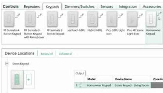
No physical keypad will get activated to this software keypad. Keep in mind that the Homeowner keypad will still consume one of the available 95 device addresses on the Clear Connect Wireless – Type A link on the RadioRA 3 processor. The main repeater and four auxiliary repeaters each consume an address, leaving 95 out of 100 addresses for devices.
