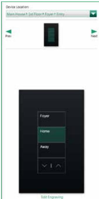
Once the button has been selected and engraved, make sure that the **Program Type** is set to **Normal** and change the **Button Type** (in the upper-middle of the screen) to **Single Action**. **Single Variable** and **Conditional** button types are considered advanced button types and cannot be edited from within the Lutron mobile app, preventing the end user from being able to apply Sonos Room control.
