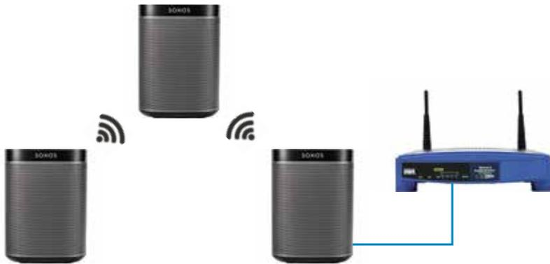
When using Boost Mode, where one Room is wired into the physical network, it is important to limit the number of hard-wired Rooms to one network. Connecting more than one Room to the network using a wired connection could cause a network loop.
