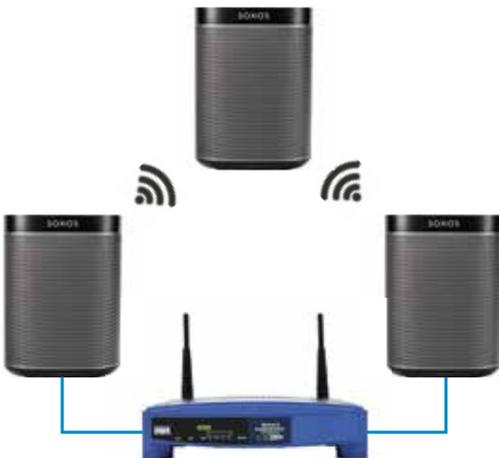
The network loop will cause broadcast and multicast commands to be repeated to all devices on the network. As network traffic builds, it will become increasingly difficult for other devices to communicate over the same network causing disruptions to all network devices.
