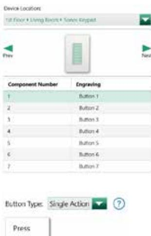
A database transfer must be performed after adding the Homeowner keypad into the system in order for it to be accessible via the Lutron mobile app.
