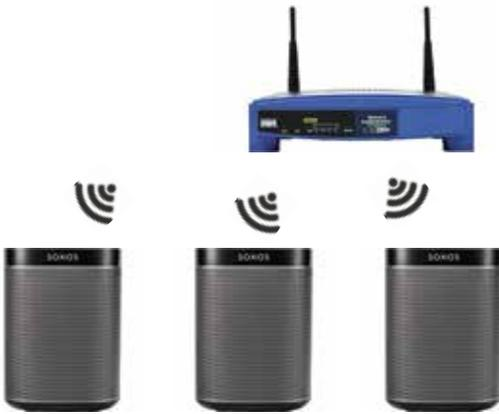
2. Boost Mode – One Room connected via wire into a router or switch and all others connected wirelessly
