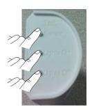
3. The device is now in channel selection mode. Cycle through the channels until you hear a beep from the repeater. Press the "Lights ON" button to try the next RF channel (15 total), the "Lights OFF" button to try the previous channel, or the Test button to retry the current channel.
