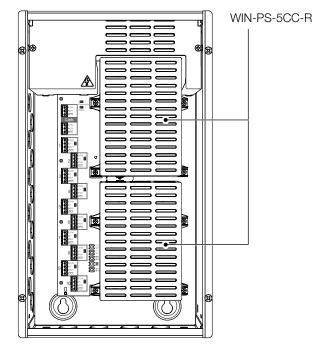
Model QSPS-10PNL with (2) power modules (WIN-PS-5CC-R) installed
