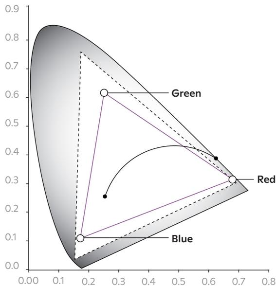
Ketra's D2 LED Downlight can easily be commissioned into Lutron HomeWorks or Athena systems. The product can reproduce any color point with the triangle shaped gamut indicated in the chart to the left. With Ketra's Color Lock tool, the color point is maintained to an accuracy of one-step MacAdam Ellipse over the lifetime of the product and across operating temperature ranges.
