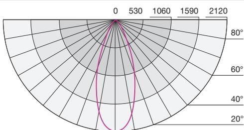
**Beam Angle: 40° Wide Flood, High Output**
