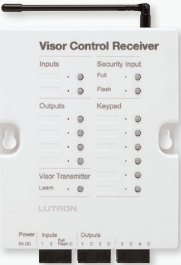
Visor control receiver RR-VCRX-WH Easy closed contact integration option
