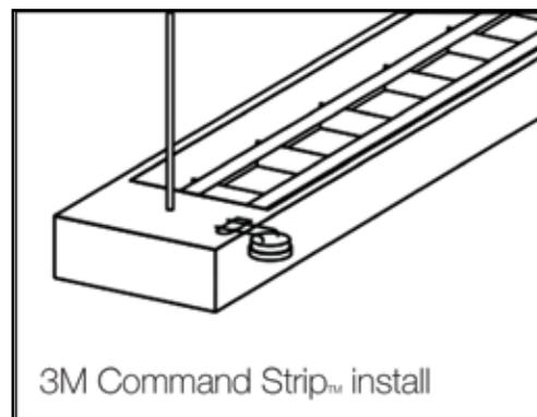
How to place the sensor on a pendant fixture using Option 3.
