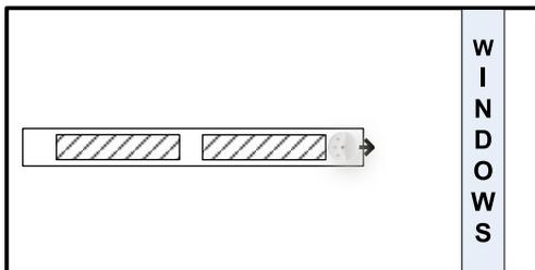
**Option 3:** You can also place the sensor in the same vertical plane as the pendant. This approach may work for pendant fixtures perpendicular to the window, depending on the fixture design.
