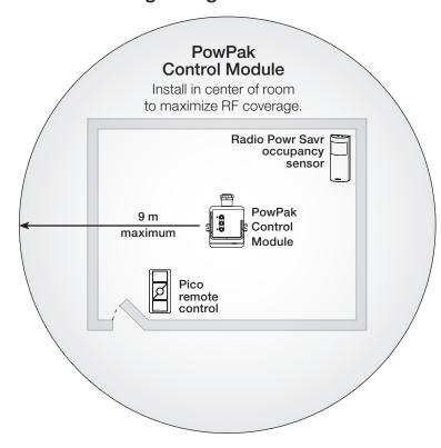
**Note:** Wireless sensors and controls must be located within 9 m of the associated control module.
