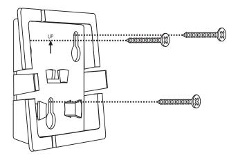
If using the DC adapter, wrap excess cord around the cord holder and snap the keypad onto the mounting bracket.
