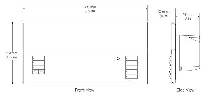
Fits into a 4-gang U.S. backbox, 90.4 mm (3.5 in) deep (Lutron P/N 245-254) or 76.2 mm (3 in) deep (Lutron P/N 241-400)
