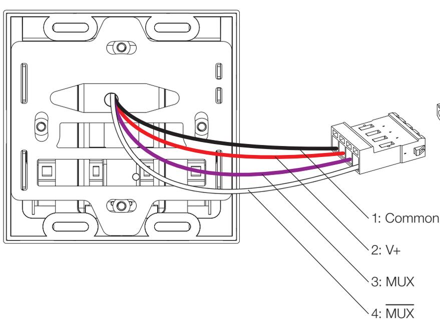
Note: Use appropriate wire-connecting devices as specified by local codes.
