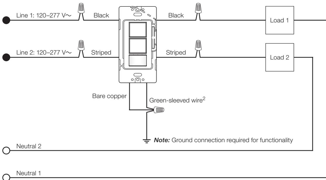
\* Wiring must comply with 2011 NEC code 210.7 for wiring Multiple Branch Circuits: Where two or more branch circuits supply devices or equipment on the same yoke, a means to simultaneously disconnect the ungrounded conductors supplying those devices shall be provided at the point at which the branch circuits originate.
