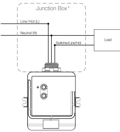
**NOTE:** Some applications (in U.S.A.) require the RF module to be installed inside an additional junction box. For information about how to perform this installation, please see Application Note #423 (P/N 048423) at www.lutron.com. Please consult all local and national electric codes for proper installation methods.
