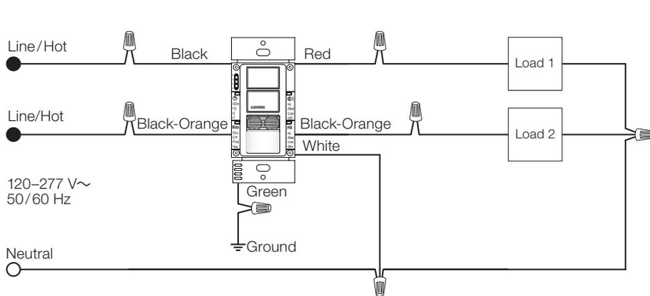
Note: When a neutral connection is available, remove green sleeve and connect the white wire to neutral.
