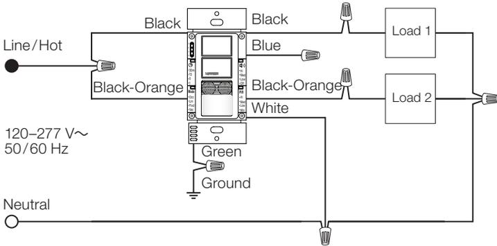
Wiring must comply with NEC® code for wiring multiple branch circuits. Where two or more branch circuits supply devices or equipment on the same yoke, a means to simultaneously disconnect the ungrounded conductors supplying those devices shall be provided at the point at which the branch circuits originate.
