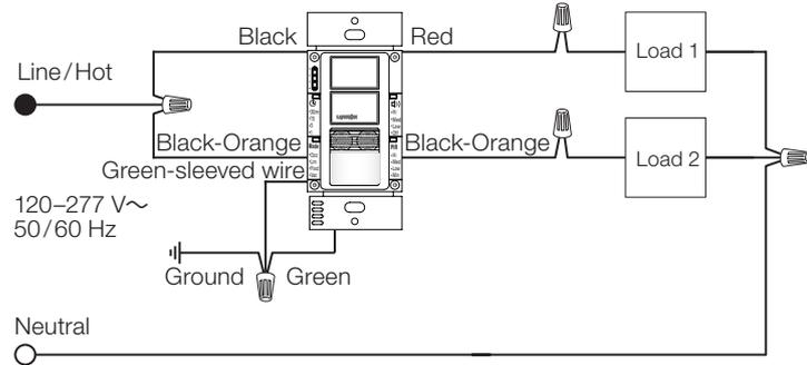
Note: Connect green-sleeved wire to ground only in retrofit and replacement applications.
