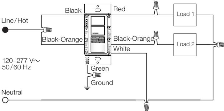
Note: When a neutral connection is available, remove green sleeve and connect the white wire to neutral.
