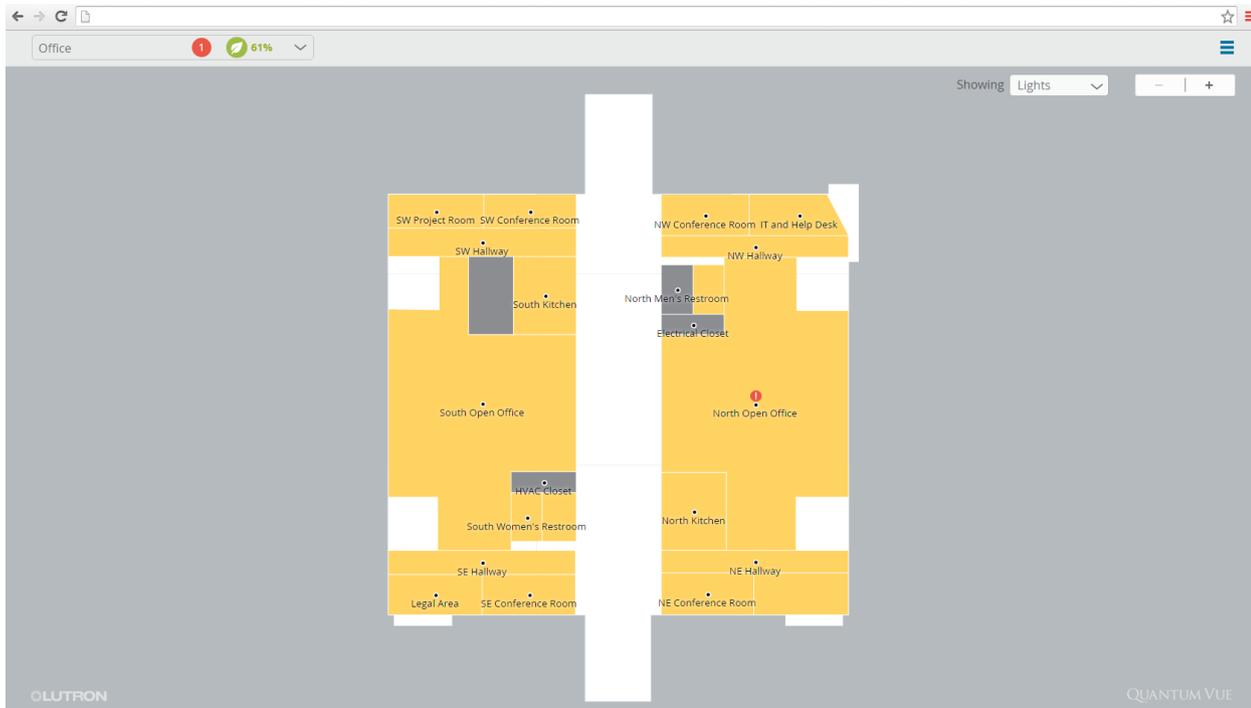
This is an example of a Quantum Vue floor plan that was created using customer supplied as-built drawings in an uneditable format (such as .pdf). The drawings contained information that cluttered the drawing and made it less intuitive so an outline of the image was used.
