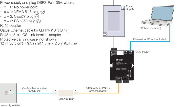
Permanently installed programming jack QS-PRG-JACK-XX-CPN7153 of myRoom™ prime system (not included)
