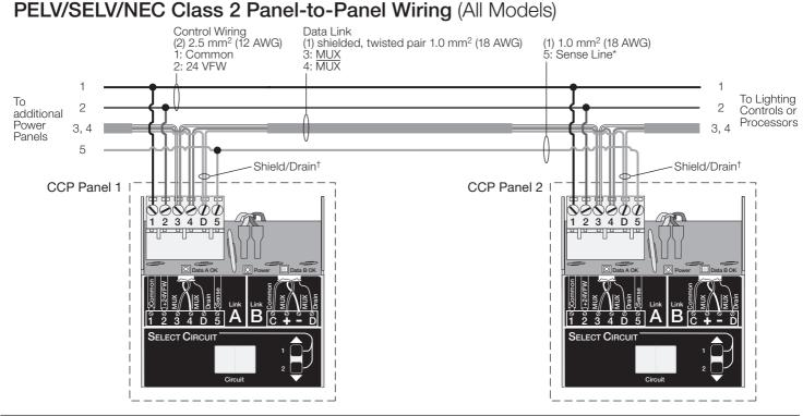
\* Emergency power: The additional 1.0 mm<sup>2</sup> (18 AWG) wire is a "sense" line from terminal 5 of another panel. This sense line allows an emergency (essential) lighting panel to "sense" when normal (non-essential) power is lost. If more than one emergency lighting panel needs to sense from a specific normal panel, a dedicated wire between each pair of normal (non-essential) and emergency (essential) panels may be required.
